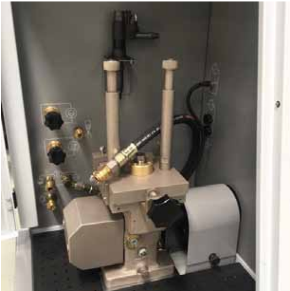
Patented Cam Box; stroke set between 10 & 18 mm.
