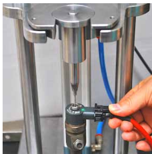
Air Gap Testing
